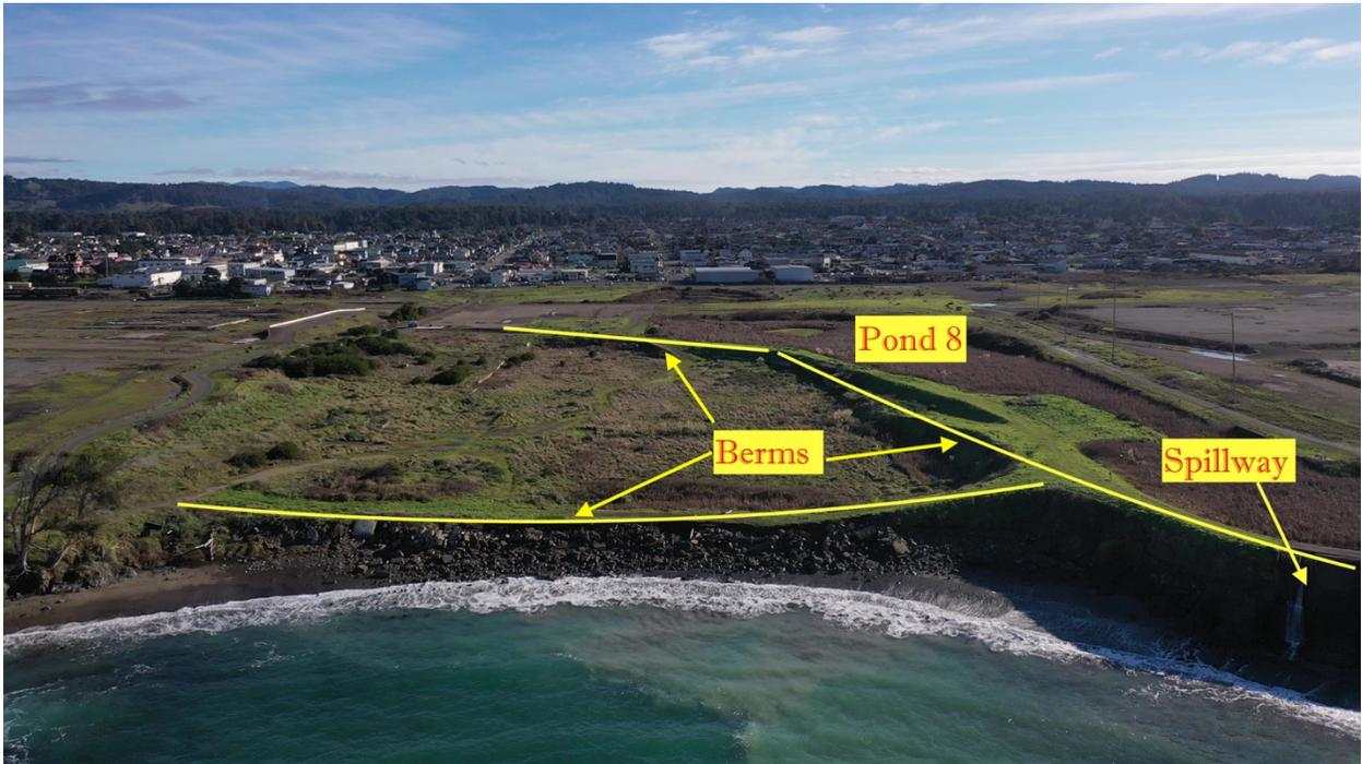
Photo 1 (with Graphics): Looking east toward downtown Fort Bragg, this aerial shot of OE-E shows that, for the time being, the ponds in this section of the old mill site, are contained by the rocks and dirt used to create the berms holding the sediments from entering the bay referred to historically as Soldier Harbor.
